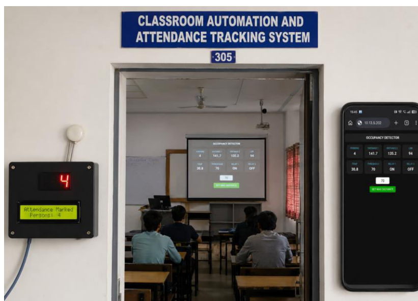
Figure.5.1. Real Time implementation of Smart Room Occupancy Detection System
